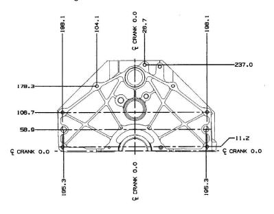
Figure 3.1.1-I: Transmission attachment
